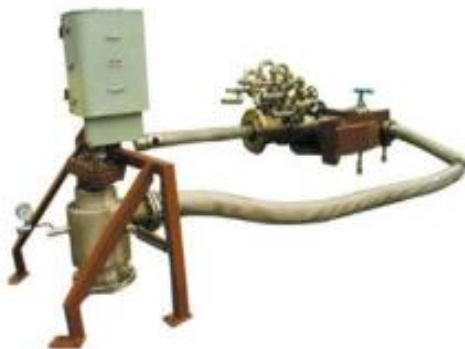
KK65T converter with water cooling, combined blowing rotary joints and gear box, main controller and encoder assembly
