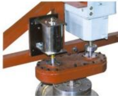
KK65T converter with water cooling, combined blowing rotary joints and gear box, main controller and encoder assembly
