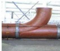
Pressure balanced compensator of the big curved tube manufactured by the compensator workshop of the company
